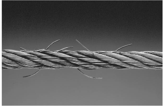
Cable With Broken Wires
